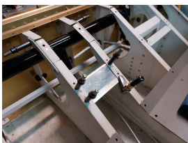
Drilled and installed the trim bracket to the seat ribs
