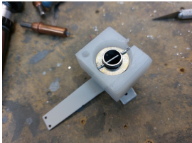
Drilled and installed the trim bracket to the seat ribs
